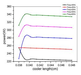
Fig. 5 Relationship between cooler length and engine power (temperature=923K)
