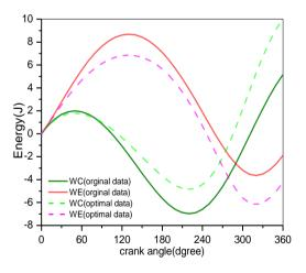
Fig. 13 Energy Variation of the compression and the expansion space
