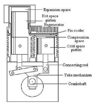
Fig. 2 gamma Stirling engine
