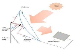
Fig. 1 Schematic diagram of solar parabolic dish system
