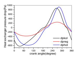
Fig. 17 Heat exchanger pressure drops virus crank angle
