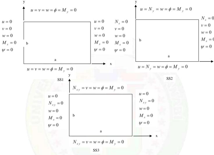
Fig. (1) Simply supported boundary conditions
