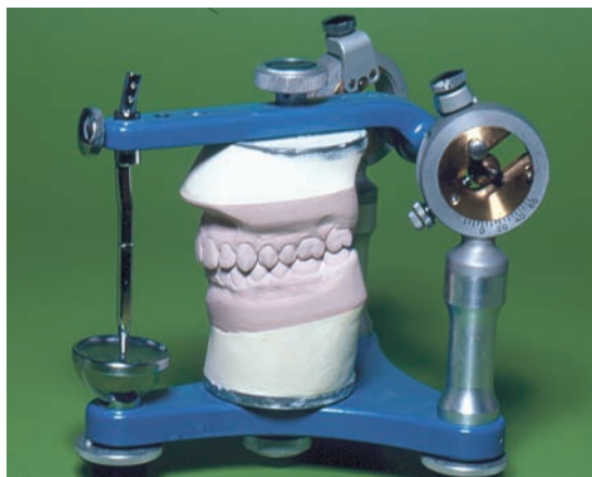
Fig. 14.5 The Dentatus ARH articulator. This is a non-Arcon instrument, with adjustable condylar angles and progressive side-shift. It has no provision for immediate side-shift.
