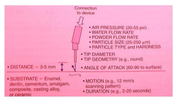
Fig-6.11 Schematic representation of range of variables associated with any type of air abrasion equipment.
