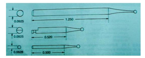
Fig-6.14 Typical dimensions (in inches) of three common instrument shank for straight handpiece, latch-angle handpiece, and friction-grip angle handpiece type
