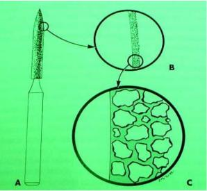
Fig-6.19 Diamond instrument construction.
