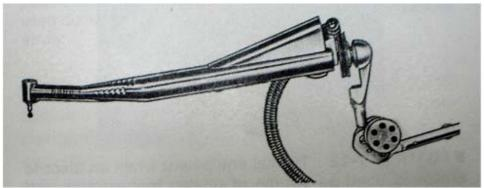
Fig-6.5 First belt-drive angle handpiece (1955) at speed > 100,000.
