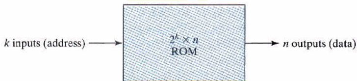
FIGURE 7.9 ROM block diagram
