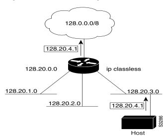
If you disable classless routing, and a router receives packets destined for a subnet of a network that has no network default route, the router discards the packet. Figure 2 shows a router in network 128.20.0.0 connected to subnets 128.20.1.0, 128.20.2.0, and 128.20.3.0. Suppose the host sends a packet to 128.20.4.1. Because there is no network default route, the router discards the packet.
