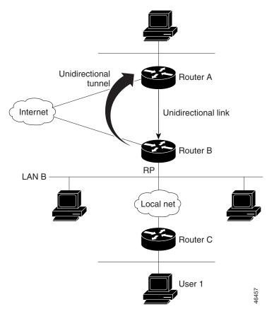
Figure 82 IGMP Mroute Proxy Mechanism
