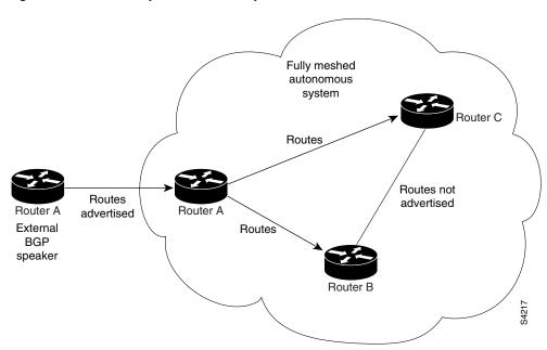
Figure 55 Three Fully Meshed iBGP Speakers
