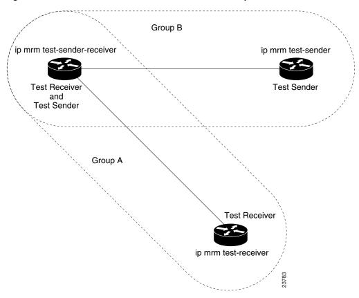
To configure the routers in Figure 86 for monitoring more than one multcast group, configure the Test Sender in Group B and the Test Receiver in Group A separately, as already discussed, and configure the following commands beginning in global configuration mode on the router or host that belongs to both Group A and Group B (in the upper left of Figure 86):
