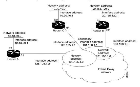
Figure 35 Disabled Split Horizon Example for Frame Relay Network
