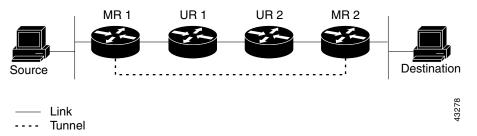
In Figure 68, Source delivers multicast packets to Destination by using MR 1 and MR 2. MR 2 accepts the multicast packet only if it believes it can reach Source over the tunnel. If this situation is true, when Destination sends unicast packets to Source, MR 2 sends them over the tunnel. Sending the packet over the tunnel could be slower than natively sending the it through UR 2, UR 1, and MR 1.
