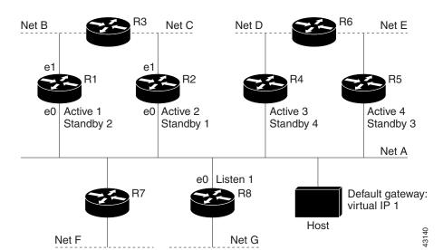
Figure 18 Network Supporting the HSRP ICMP Redirection Filter
