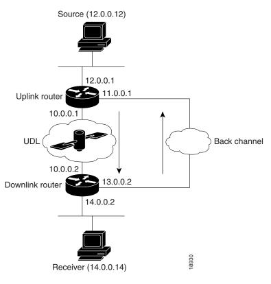
Figure 84 IGMP Unidirectional Link Routing Example
