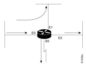
A directed broadcast address includes the network or subnet fields. For example, if the network address is 128.1.0.0, the address 128.1.255.255 indicates all hosts on network 128.1.0.0, which would be a directed broadcast. If network 128.1.0.0 has a subnet mask of 255.255.255.0 (the third octet is the subnet field), the address 128.1.5.255 specifies all hosts on subnet 5 of network 128.1.0.0—another directed broadcast.
