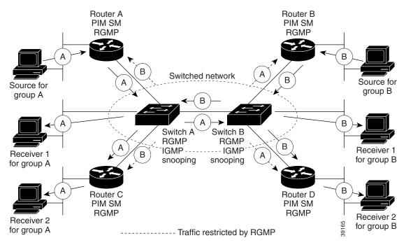
Figure 89 RGMP in a Switched Network
