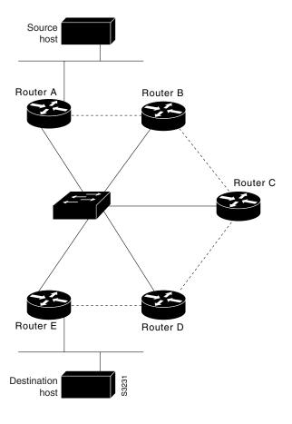
Figure 10 Physical Configuration of a Sample NBMA Network
