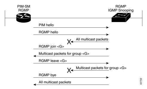
The router sends simultaneous PIM hello (or a PIM query message if PIM Version 1 is configured) and RGMP hello messages to the switch. The PIM hello message is used to locate neighboring PIM routers. The RGMP hello message instructs the switch to restrict all multicast traffic on the interface from which the switch received the RGMP hello message.
