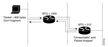
IP Path MTU Discovery is useful when a link in a network goes down, forcing the use of another, different MTU-sized link (and different routers). As shown in Figure 17, suppose a router is sending IP packets over a network where the MTU in the first router is set to 1500 bytes, but the second router is set to 512 bytes. If the "Don't fragment" bit of the datagram is set, the datagram would be dropped
