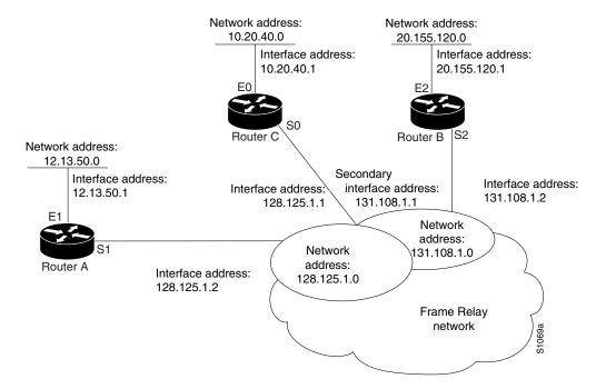
In this example, split horizon must be disabled in order for network 128.125.0.0 to be advertised into network 131.108.0.0, and vice versa. These subnets overlap at Router C, serial interface 0. If split horizon were enabled on serial interface 0, it would not advertise a route back into the Frame Relay network for either of these networks.
