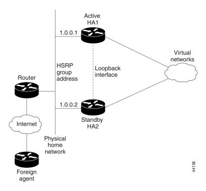
Figure 32 Topology Showing HA Redundancy on Multiple Virtual Networks Using One Physical Network (Same Subnet)
