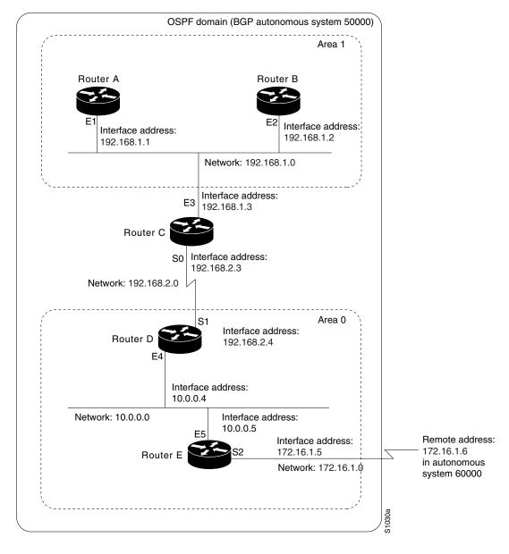
Figure 63 Example OSPF Autonomous System Network Map
