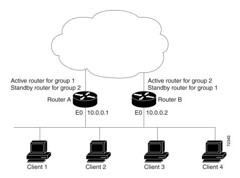
The following example shows Router A configured as the active router for group 1 with a priority of 110 and Router B configured as the active router for group 2 with a priority of 110. The default priority level is 100. Group 1 uses a virtual IP address of 10.0.0.3 and Group 2 uses a virtual IP address of 10.0.0.4.
