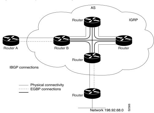
Figure 59 BGP Synchronization Configuration
