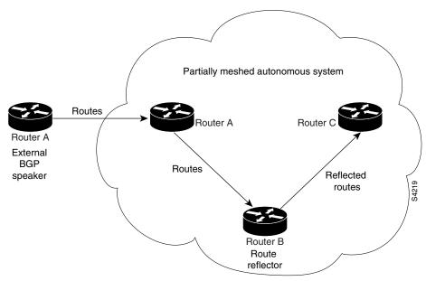
Figure 56 Simple BGP Model with a Route Reflector
