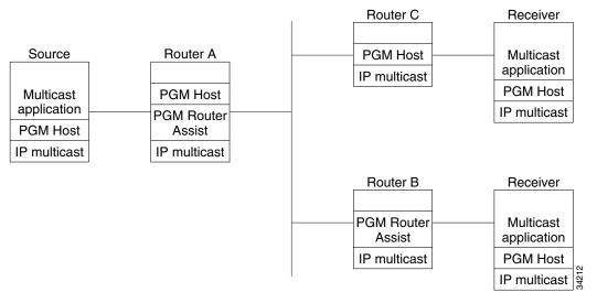
When the router is functioning as a network element (PGM Router Assist is configured) and PGM Host is configured (Router A in Figure 81), the router can process received PGM packets as a virtual PGM Host, originate PGM packets and serve as its own first hop PGM network element, and forward received PGM packets.
