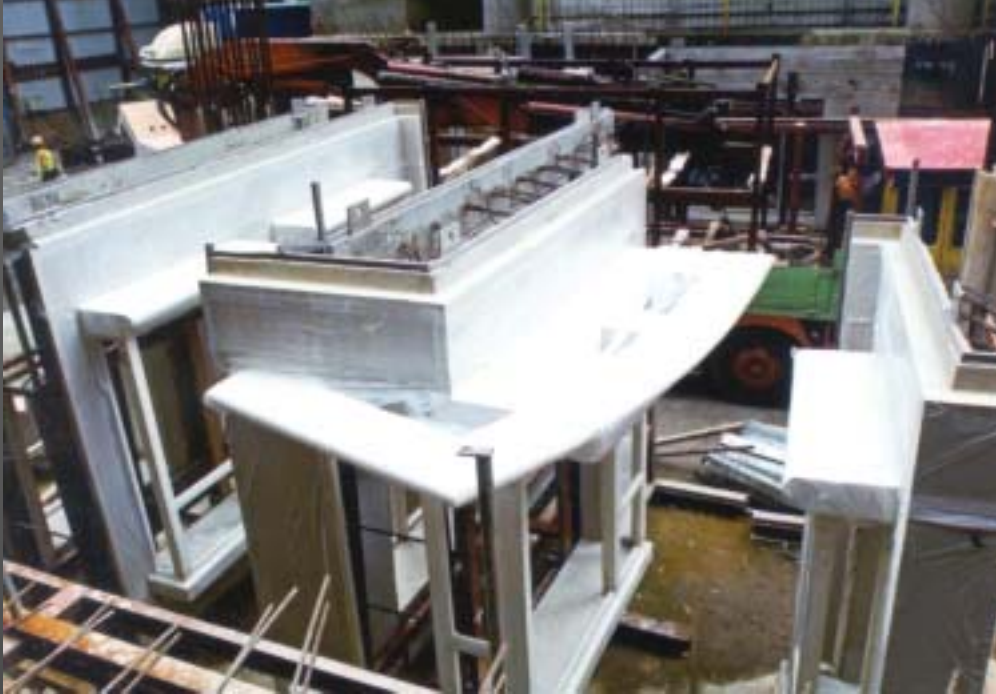
Detail of the precast balcony unit
